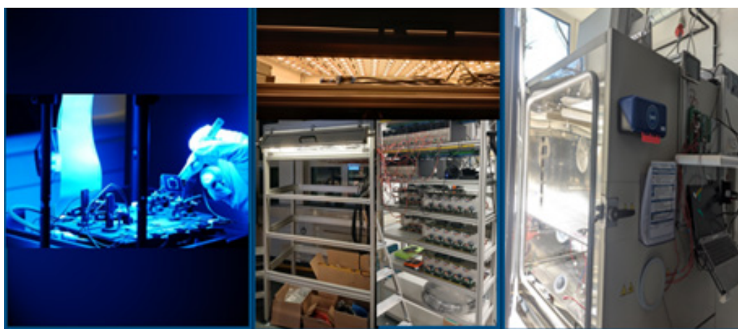
Tandem-compatible indoor accelerated testing Light, T, cycles (N 2 /air)
